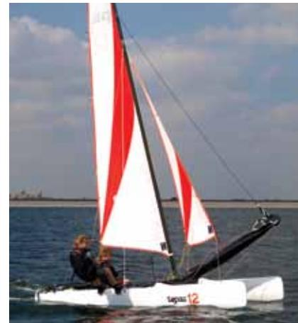
**ABOVE** Halyards can be tucked away neatly at the foot of the mast leaving the trampoline uncluttered
