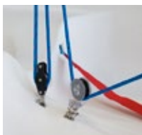
Possibility to put in a ratchet block to create a regatta mainsheet system.
